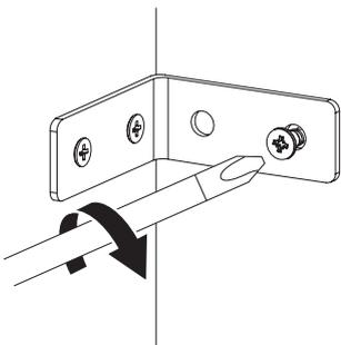
When you are happy with the position of the cabinet, using suitable wall fixings (not supplied), fix the cabinet to the wall through the brackets.
