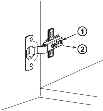
Remove any doors as shown, pushing the clip to the rear of each hinge and lifting away from the base plate. Make sure the door is supported when unclipping each hinge.
